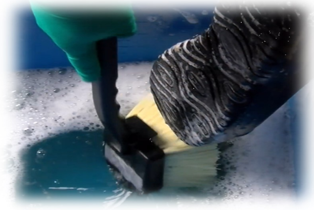
Figure 2: Pay special attention to scrubbing the threads with soap and water to remove all debris.
